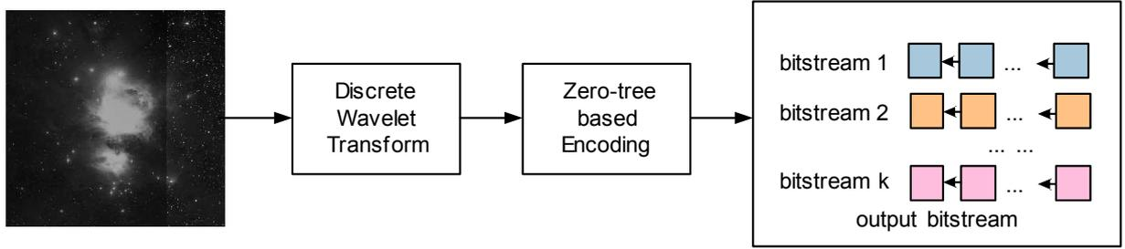
Figure 1. Procedure of wavelet compression for astronomical images
