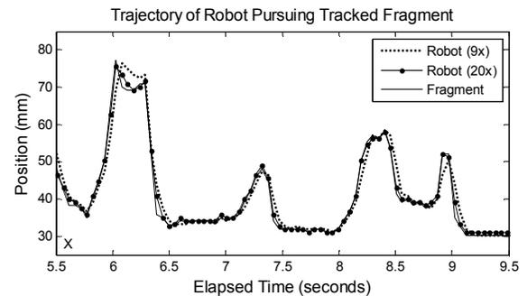
Fig. 7. Close-up view of Fig. 5 and Fig. 6 superimposed, illustrating the increased ability of the robot to follow a reduced speed target.
