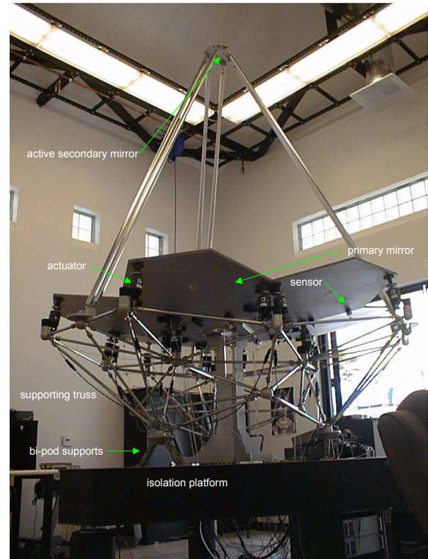
Figure 1: SPACE testbed
